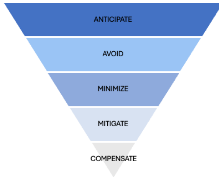
Figure 4.1. Mitigation hierarchy framework for risk assessment in the context of an ERW project.
